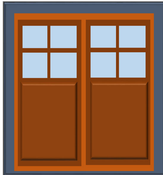
Fig 4.14: Partly paneled window
