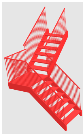
Fig 4.32 (a): Quarter-turn Staircase
