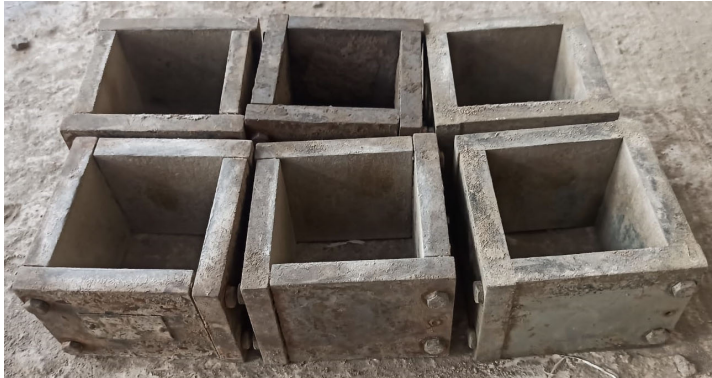
Fig. 6.5: Moulds for preparing cement mortar cubes (each face with area 50 \text{ cm}^2 )
