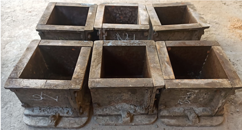
Fig. 6.18: Moulds for preparing concrete cubes (150 mm side)
