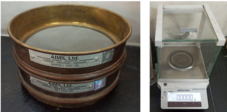
Fig. 6.1: (a) IS sieve of size 90 microns with pan, (b) Digital weighing balance
