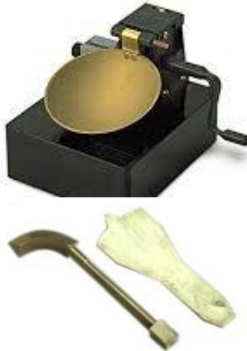
Casagrande's liquid limit apparatus and grooves
